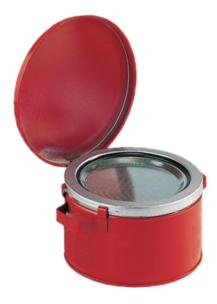
Dimensions: 120 x 130 ( dia x H in mm), interior tin-plated, exterior red powder coated, flame arrester as soaking tray, Marking prepared according to GefStoffV and BGV A8. testing: FM-tested
