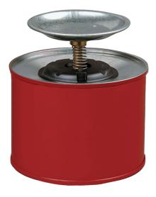
Dimensions:  $180 \times 190$  ( dia x H in mm). Soaking tray: 135 mm dia, interior tin plated, exterior red powder coated, soaking tray with flame arrester, brass pump tube and PPS. Marking prepared according to GefStoffV and BGV A8. testing: FM-tested
