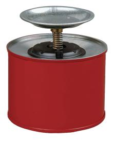
Dimensions: 180 x 190 ( dia x H in mm). Soaking tray: 135 mm dia, interior tin plated, exterior red powder coated, soaking tray with flame arrester, brass pump tube and PPS. Marking prepared according to GefStoffV and BGV A8. testing: FM-tested
