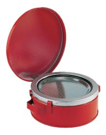
Dimensions:approx. 240  $\times$  100 ( dia  $\times$  H in mm), interior tin-plated, exterior red powder coated, flame arrester as soaking tray, Marking prepared according to GefStoffV and BGV A8. testing: FM-tested
