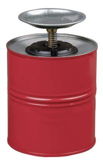
Dimensions:  $180 \times 270$  ( dia x H in mm). Soaking tray: 135 mm dia, interior tin plated, exterior red powder coated, soaking tray with flame arrester, brass pump tube and PPS. Marking prepared according to GefStoffV and BGV A8. testing: FM-tested
