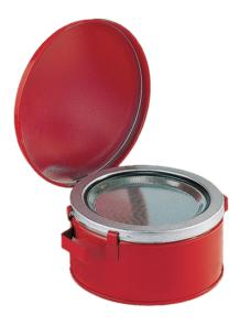
Dimensions:approx. 240  $\times$  120 ( dia  $\times$  H in mm), interior tin-plated, exterior red powder coated, flame arrester as sooking tray, Marking prepared according to GefStoffV and BGV A8. testing: FM-tested
