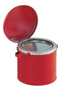
Dimensions: 290 x 270 (dia x H in mm), interior tin-plated, exterior red powder coated, flame arrester as soaking tray, Marking prepared according to GefStoffV and BGV A8, testing: FM-tested
