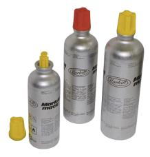
Pure aluminium bottle, break-proof, screw cap red dim: 60 x 220 (dia x H in mm), automatic pouring and venting valve, self-closing pouring valve opens only by finger pressure, automatic closing when not in use - even without srew cap. Interior seal from Viton. testing: RWTÜV-tested
