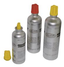
Pure aluminium bottle,break-proof,screw cap yellow dim: 78 x 280 (dia x H in mm) automatic pouring and venting valve, self-closing pouring valve opens only by finger pressure, automatic closing when not in use - even without srew cap. Interior seal from EPDM testing: RWTÜV-tested
