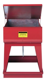
capacity: approx. 48 litres outside dimensions: 610 x 496 x 845 (WxDxH) mm basin (inside): 603 x 406 x 222 (WxDxH) mm Basin, lid and frame made from galvanised sheet steel, red coated. "3/4""drain plug in basin bottom for" selective emptying. Slow, independent closing of the lid via pneumatic cylinder. Testing: FM-approved
