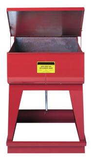
capacity: approx. 48 litres outside dimensions:  $610 \times 496 \times 845$  (WxDxH) mm basin (inside):  $603 \times 406 \times 222$  (WxDxH) mm Basin, lid and frame made from galvanised sheet steel, red coated. "3/4""-drain plug in basin bottom for" selective emptying. Slow, independent closing of the lid via pneumatic cylinder. Testing: FM-approved
