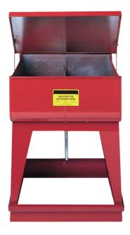
capacity: approx.  $2 \times 15$  litres outside dimensions:  $610 \times 496 \times 845$  mm (W x D x H) basin (inside):  $2 \times 298 \times 406 \times 140$  mm(W x D x H) Basin, lid and frame made from galvanised sheet steel, red coated. For cleaning of extremely contaminated components. 1. chamber: pre-cleaning, 2. chamber: final cleaning "3/4""- drain plug in basin bottom for selective emptying. Testing: FM-approved
