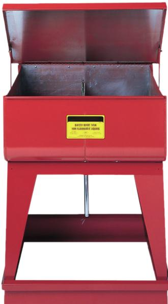
capacity: approx. 2 x 15 litres outside dimensions: 610 x 496 x 845 mm (W x D x H) basin (inside): 2x 298 x 406 x 140 mm(W x D x H) Basin, lid and frame made from galvanised sheet steel, red coated. For cleaning of extremely contaminated components. 1. chamber: pre-cleaning, 2. chamber: final cleaning "3/4"- drain plug in basin bottom for selective emptying. Testing: FM-approved
