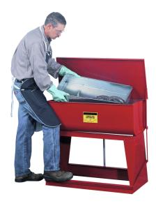
capacity: 97 litres outside dimensions:  $895 \times 496 \times 845$  (WxDxH) mm basin (inside):  $899 \times 406 \times 305$  (WxDxH) mm Basin, lid and frame made from galvanised sheet steel, red coated. "3/4""- drain plug in basin bottom for" selective emptying. Slow, independent closing of lid via pneumatic cylinder. testing:
