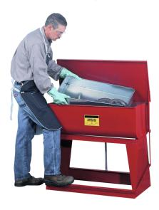
capacity: 97 litres outside dimensions: 895 x 496 x 845 (WxDxH) mm basin (inside): 899 x 406 x 305 (WxDxH) mm Basin, lid and frame made from galvanised sheet steel, red coated. "3/4""- drain plug in basin bottom for" selective emptying. Slow, independent closing of lid via pneumatic cylinder. testing:
