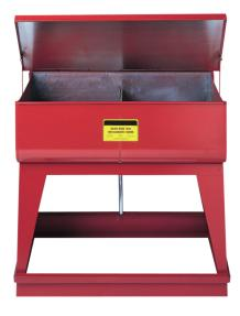
capacity: approx. 2 x 34 litres Outside dimensions: 895 x 496 x 845 mm (WxDxH) basin (inside):  $2x438 \times 406 \times 222$  mm (WxDxH) Basin, lid and frame made from galvanised sheet steel, red coated. For cleaning of extremely contaminated components. 1. chamber: pre-cleaning, 2. chamber: final purification. "3/4""- drain plug in bottom of each chamber" for selective emptying. Testing: FM-approved
