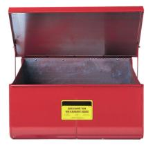
capacity: approx. 48 litres outside dimensions: 610 x 496 x 273 mm (W x D x H) basin (inside): 603 x 406 x 273 mm (W x D x H) For positioning on a workbench. Basin and lid made from galvanised sheet steel, red coated. self-closing lid in case of fire "3/4""- drain plug in basin bottom for" selective emptying. Testing: FM-approved
