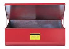
capacity:approx. 97 litres outside dimensions: 895 x 496 x 336 mm (W x D x H) basin (inside): 889 x 406 x 336 mm (W x D x H) For positioning on a workbench. Basin, lid and frame made from galvanised sheet steel, red coated. self-closing lid in case of fire "3/4""- drain plug in basin bottom for" selective emptying Testing: FM-approved
