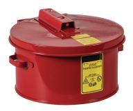
Dim:approx. 240 x 160 (dia x H in mm), outside: powder coated red, inside: tin-plated, self-closing lid in case of fire, via safety fuse. Markings prepared according to GefStoffV and BGV A8 testing: FM/ UL- tested
