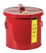
Dim:approx. 300 x 310 (dia x H in mm), outside:powder coated, red, inside:tin-plated, self-closing lid in case of fire via safety fuse. Markings prepared according to GefStoffV and BGV A8 testing: FM/UL- tested
