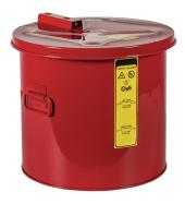
Dim:approx. 360 x 360 (dia x H in mm), outside:powder coated, red, inside:tin-plated, Self-closing lid in case of fire via safety fuse. Markings prepared according to GefStoffV and BGV A8 testing: FM/UL- tested
