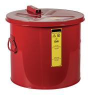
Dim:  $410 \times 390$  (dia x H in mm), outside: powder coated, red,inside:tin-plated inside: tin-plated, self-closing lid in case of fire via safety fuse. Markings prepared according to GefStoffV and BGV A8 testing: FM/ UL- tested
