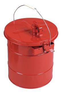
Dim:  $380 \times 405$  ( dia x H in mm ), capacity: 19 litres, sheet steel interior tin-plated , exterior red powder coated, self closing filling opening with flame arrest, secure closing lid, automatic pressue compensation, with earthing jumper.
