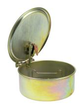
Capacity: 2 I Dim. approx.: 230 x 100 (Dia x H ) mm Self-closing lid in case of fire via fuse Marking prepared according to GefStoffV and BGV A8
