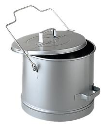
for non-flammable liquids dimensions: 310  $\times$  260 (Dia  $\times$  H) mm sheet steel, hot-dip galvanised with apportionable carrying handle Marking prepared meeting GefStoffV and BGV A8 Testing: GS-sign
