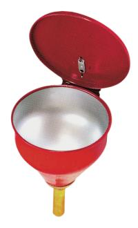
with imerstion tube act as flame arrester Filling opening dia: 280 mm Length of flame arrester: 150 mm funnel exterior red powder coated interior tin plated immersion tube and flame arrester made from brass, 2 " thread Self-closing lid in case of fire via fusible Testings: FM-approved
