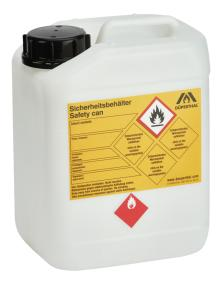
Colour: white, transparent Dimensions:  $191 \times 149 \times 256$  (L x W x H mm) Fill diameter: approx. 56 mm Screw cap (type S 60/61) Approval: UN 3H1/Y1.9/200/...A/PA-03/48248/SIS Note: In order to guarantee tight closure of the canister, it has to be closed with a torque of 20 Nm. For this purpose, we recommend our special pliers, ref. 5.09.003.
