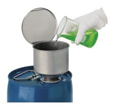
for art. 5.10.006 and 5.10.010 Filler opening dia 120 mm Buttress thread S 56x4 overfilling protection, hinged lid, PE sealing flame arrester stainless steel (changeable) earthing chain ring for in connection with a canister will a prevents overfilling Markings according to GefStoffV and BGV A8
