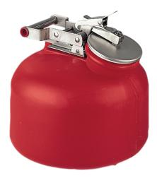
Dimension: 310 x 350 (Dia x H in mm) Self-Closing lid, lockable large filling opening 90 mm dia fittings made from galvanised sheet steel, Earthing connection in handel connected to flame arrester in neck Marking prepared to GefStoffV and BGV A8 Testing: tested by FM
