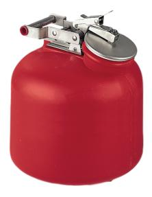
Dimension: 310 x 450 (Dia x H in mm) Self-Closing lid, lockable large filling opening 90 mm dia fittings made from galvanised sheet steel, Earthing connection in handel connected to flame arrester in neck Marking prepared to GefStoffV and BGV A8 Testing: tested by FM
