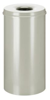
dim: 335 x 625 (dia x H mm), capacity approx. 50 l container and extinguishing head made from steel, light grey RAL 7035, Extinguisher head design prevents supply of oxygen in case of fire.
