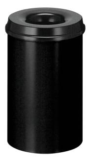
dim: 260 x 426 (dia x H mm) container and extinguishing head made from steel, black RAL 9011, Extinguisher head design prevents supply of oxygen in case of fire, testing: GS-sign
