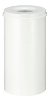
dim: 335 x 625 (dia x H mm) container and extinguishing head made from steel, white RAL 9002, Extinguisher head design prevents supply of oxygen in case of fire.
