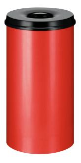
dim: 335 x 625 (dia x H mm) container and extinguishing head made from steel, extinguisher head black RAL 9011, extinguisher body red RAL 3000, Extinguisher head design prevents supply of oxygen in case of fire.
