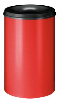
dim:  $450 \times 710$  (dia x H mm) container and extinguishing head made from steel, extinguisher head black RAL 9011, extinguisher body red RAL 3000, Extinguisher head design prevents supply of oxygen in case of fire.
