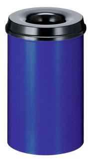
dim: 260 x 426 (dia x H mm) container and extinguishing head made from steel, extinguisher head black RAL 9011, extinguisher body blue RAL 5013, Extinguisher head design prevents supply of oxygen in case of fire, testing: GS-sign
