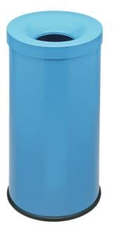
dim: 450 x 710 (dia x H mm) container and extinguishing head made from steel, extinguisher head black RAL 9011, extinguisher body blue RAL 5013, Extinguisher head design prevents supply of oxygen in case of fire.
