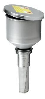
Filler opening 120 mm dia, with G2 " pipe thread (G2 " bushing with 2 " Tri-Sure-buckler) incl. viton-seal, overfill-protection, flap lid. For use ONLY with flame arrester: Article 5E10.004 or 5.88.003 in this combination an overfill is not possible, Marking prepared according to GefStoffV and BGV A8
