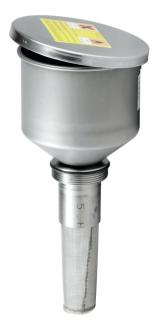
Filler opening 120 mm dia, with G2 " pipe thread (G2 " bushing with 2 " Tri-Sure-buckler) incl. viton-seal, overfill-protection, flap lid. For use ONLY with flame arrester: Article 5E10.004 or 5.88.003 in this combination an overfill is not possible, Marking prepared according to GefStoffV and BGV A8
