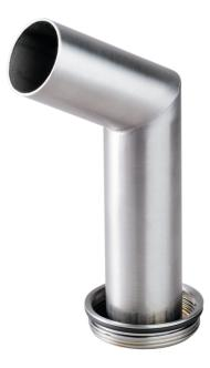
insertable with article 5.88.003, appropriate for ref. no. 5.88.010/5.88.110, discharge opening dia: 40 mm length: 160 mm (curved)
