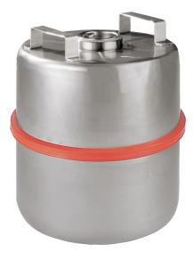
Stainless steel, 1.4571 unpolished, Dim:  $280 \times 290$  (dia x H) mm, 2" thread including Tre-sure plug with viton-seal without flame arrester. Marking prepared according to GefStoffV and BGV A8
