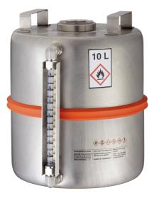
stainless steel, 1.4571 unpolished, Dim: 280 x 290 (dia x H) mm, level indicator made from PFA, 2" thread including Tre-sure plug with viton seal without flame arrester. Marking prepared according to GefStoffV and BGV A8
