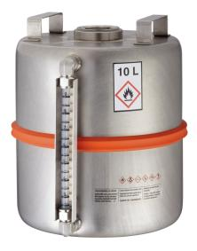
stainless steel, 1.4571 unpolished, Dim:  $280 \times 290$  (dia x H) mm, level indicator made from PFA, 2" thread including Tre-sure plug with viton seal without flame arrester. Marking prepared according to GefStoffV and BGV A8
