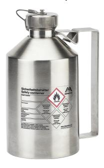
Stainless steel 1.4571 (AISI 316Ti) polished Dimensions: approx. 100 x 210 mm (dia x H) Seals: LDPE Closes tightly, captive cap on flexible shaft including cap locking mechanism. Flame arrester in container neck. Markings prepared according to GefStoffV and Workplace Directive A1.3 (ASR).
