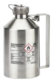
Stainless steel 1.4571 (AISI 316Ti) polished Dimensions: approx. 100 x 210 mm (dia x H) Seals: LDPE Closes tightly, captive cap on flexible shaft including cap locking mechanism. Flame arrester in container neck. Markings prepared according to GefStoffV and Workplace Directive A1.3 (ASR).
