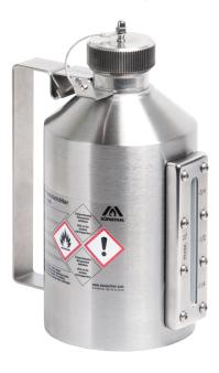
Stainless steel 1.4571 (AISI 316Ti) polished Dimensions: approx. 100 x 210 mm (dia x H) Seals: LDPE Dimensions: approx. 100 x 210 mm (dia x H) Closes tightly, captive cap on flexible shaft including cap locking mechanism, Flame arrester in container neck, measuring scale, Markings prepared according to GefStoffV and Workplace Directive A1.3 (ASR).
