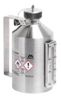
Stainless steel 1.4571 (AISI 316Ti) polished Dimensions: approx. 100 x 210 mm (dia x H) Seals: LDPE Dimensions: approx. 100 x 210 mm (dia x H) Closes tightly, captive cap on flexible shaft including cap locking mechanism, Flame arrester in container neck, measuring scale, Markings prepared according to GefStoffV and Workplace Directive A1.3 (ASR).
