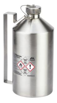
Stainless steel 1.4571 (AISI 316Ti) polished Dimensions: approx. 120 x 270 mm (dia x H) Seals: LDPE Closes tightly, captive cap on flexible shaft including cap locking mechanism, Flame arrester in container neck, Markings prepared according to GefStoffV and Workplace Directive A1.3 (ASR).
