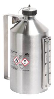
Stainless steel 1.4571 (AISI 316Ti) polished Dimensions: approx. 120 x 270 mm (dia x H) Seals: LDPE Closes tightly, captive cap on flexible shaft including cap locking mechanism, Flame arrester in container neck, Level control via integrated sight glass with measuring scale, Markings prepared according to GefStoffV and Workplace Directive A1.3 (ASR).
