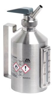
Stainless steel 1.4571 (AISI 316Ti) polished Dimensions: approx.  $100 \times 210 \text{ mm}$  (dia x H) without srew cap. Flame arrester in container neck, Level control via integrated sight glass with measuring scale. Markin prepared according to GefStoffV including self-closing metering tap with seal of PTFE. Open by pushing or pulling. Self-closing prevents uncontrolled leakage of liquids. Setting ring for adjustment, afeter installation vertically adjustable.
